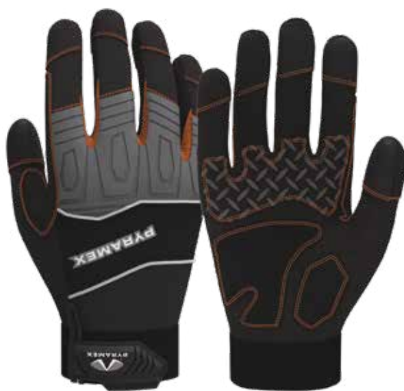
GL102 EN388: 2003 – 3241 Synthetic leather + silicone patches // Spandex plus mesh fabric on back // Embossed neoprene on knuckle // Hook + loop closure // Touchscreen capability GL102 S – 2XL
