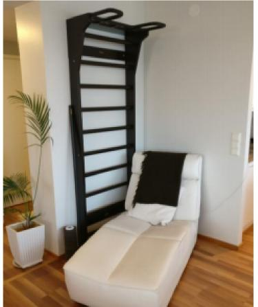
Lift the Wall Bars to its correct place. Ensure that you have marked the correct location for the fastening wooden mounting rails. Also, make sure to use proper and safe connection to studs or other type of wall structure.
