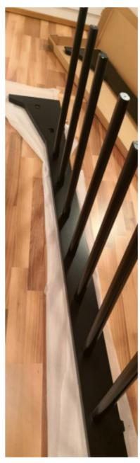
Cover the floor so that the floor or Wall Bars will not get scratches. Lay the first long wooden side rail on the floor.
