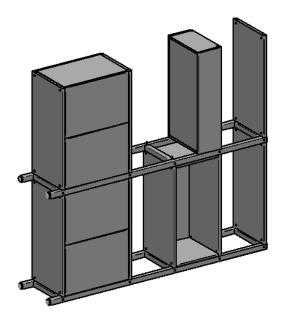
Attached lower storage unit, planter box and shelf. Note: Attach planter box to the mid-frame using M6 x 25 bolts.
