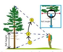
Stand at a distance approximately as far away from the object and the object's height for best results. The reference height mark should be set at 2 meters/6feet.
