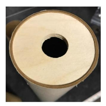
6. With the cone laying horizontally on your work surface mix up some medium cure epoxy. Drizzle epoxy a good half way down the cone rotating it. We want to ensure there is enough epoxy to run down securing the 3" HD MMT to the plastic. Insert the 3" HD MMT into the ring and down as far as the tube will go. Stand the cone up with the forward end facing the ground and allow the epoxy to run down and cure.
