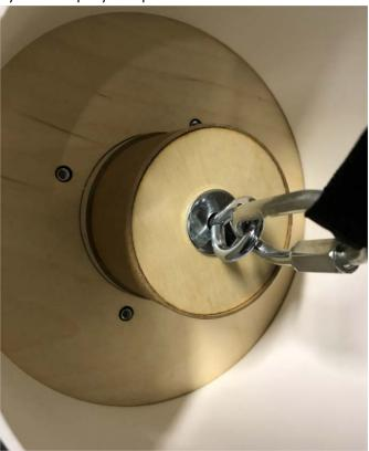
9. Attach quick link to tubular nylon loop. Thread through other 3" coupler attaching to the nose weight module's eye bolt. As show above. Insert nose weight into 3" HD MMT.
