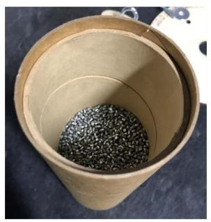
When satisfied with amount of weight to be used, epoxy in place in the stiffy. Allow to cure. Insert bulkhead and eye bolt – epoxy into place.
