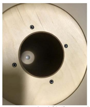
You may also epoxy the end of the 3" HD MMT to the mounting right inside the T nuts for added strength.
