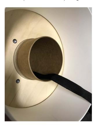
11. Thread end of tubular nylon through the hole in the top mount ring. Screw the top mount ring into place.
