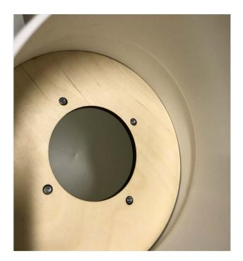
4. Pull the ring toward the cone shoulder until the ring is flush. When satisfied with the fit epoxy the ring into place bonding the ring to the cone. Forward and aft ends are OK to do currently. Don't get any epoxy in the T nuts!!!
