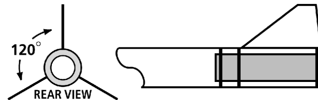
CROSS SECTION OF CENTERING RINGS/ MOTOR MOUNT TUBE ASSEMBLY IN MAIN AIRFRAME.
