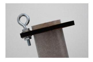
You may optionally mix a small amount of epoxy and apply it to the top and bottom nuts to prevent them from backing out.
