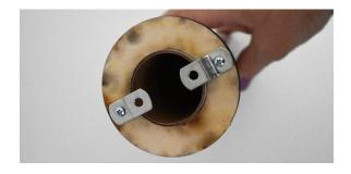
Remove the Z-clips for now to avoid accidental epoxying in place. Ensure the aft centering ring hasn't moved. Prepare a small amount of epoxy and then, using a popsicle stick, apply a fillet to the *lower side* of the aft centering ring. Make absolutely certain that no epoxy drips into the T-nuts.
