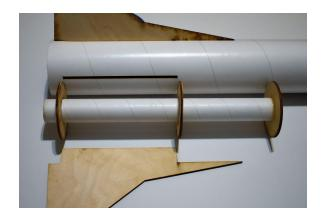
Remove the fin used for spacing and then prepare a small amount of epoxy. Using a popsicle stick, apply a fillet to the *upper side* of the middle centering ring. Let this fully cure before moving on to the next step.
