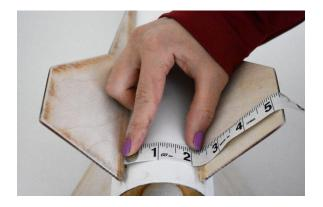
Again with a ruler, draw a straight line up your rocket's body tube between and extending beyond the two points. From the bottom of the rocket, mark points at 3 and 12 inches along this line. These points will be the locations of the rail guides.
