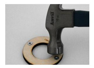
The screws and Z-clips will screw into the underside of this centering ring in later steps and for motor retention.
