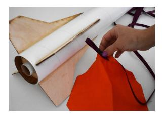
With the parachute starting laid out flat, align the shroud lines such that you have a loop at one end and the parachute at the other end. At roughly 1/3 of the length of the exposed shock cord, from the free end, attach the parachute to the shock cord with a lark's foot knot. This is done by passing the parachute canopy around the shock cord and then through the shroud line loop.
