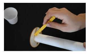
Once the epoxy bonds on the forward ring have cured, you may move on to the middle and bottom centering rings.
