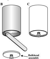
**B)** Spread a layer of epoxy around the inside circumference of the coupler to a depth of about 1/2". **C)** Push the bulkhead assembly into
