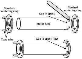
Spread a bead of epoxy around the circumference of one end of the motor tube leaving a 1" gap in the bead for the notch in the centering ring. Slip the notched centering ring over the motor tube with the notch aligned with the gap in the epoxy bead. Be sure the notch in the ring remains clear of epoxy. Locate the ring 1/2" from the end of the motor tube and allow the epoxy to set. Apply an epoxy fillet to each side of the ring still keeping the notch clear.
