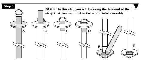
*A)* Pull the free end of the strap through the slot in the piston bulk plate.
