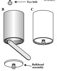
B) Spread a layer of epoxy around the inside circumference of the coupler to a depth of about 1/2".
