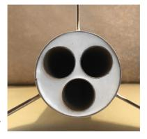
exposed to one end. Allow to cure. Insert each bulkhead in opposite ends of the coupler tube. The baffle tubes will be next to each other. Check fit, once satisfied you can epoxy in place. Epoxy one side at a time give the FWD and AFT of the bulkhead an epoxy fillet to the coupler to ensure strength.
