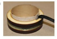
excess cord. Recess so you have sufficient space to epoxy ring into airframe. Install other ring on opposite end flush. Epoxy fillet the void between the rings, soaking the shock cord. Be careful **NOT TO** get any epoxy on the OD of the rings. Allow to cure.
