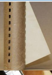
**STEP 1** The booster has been laser marked for easy glassine removal. With a hobby knife, lift up a section of the outer coating, one or two layers and peel away. This is in preparation for the fiberglass to be applied. Peel each section one at a time. Sand smooth once finished.
