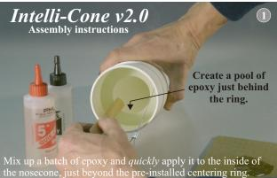
Mix up a batch of epoxy and *quickly* apply it to the inside of the nosecone, just beyond the pre-installed centering ring. Scoop it up with a stick and scrape it off against the edge of the ring allowing it to run down the back side and pooling there.
