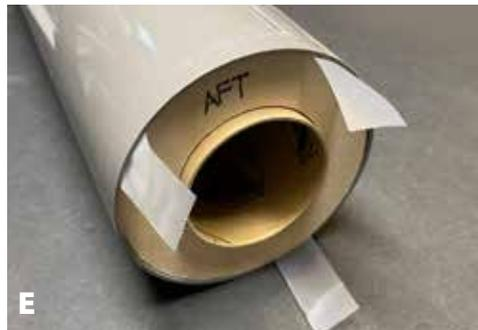
**E. Dry fit**/test the fit of the aft ring over the motor tube. You need to be able to slip this ring on and off during final motor tube/airframe assembly.
