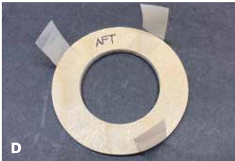
**D.** Remove the motor retainer from the motor tube. Make three or four cellophane tape tabs as shown above to aid in removing this ring at a later step.
