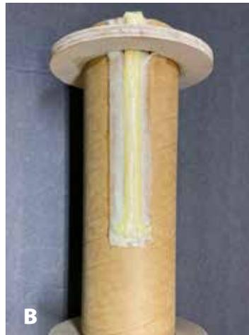
notch and press it firmly into the epoxy on the side of the motor tube. Hold the strap in place against the tube with masking tape until the epoxy cures. When cured, remove the masking tape.
