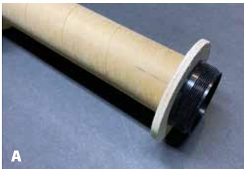
**A.** Slip the MID then AFT centering ring over the motor tube. Then **dry fit** (NO EPOXY!) the motor retention ring onto the motor tube. Make sure the retention ring is all the way onto the motor tube (approx. 3/8"). Slip the AFT ring down so it butts up against the retention ring
