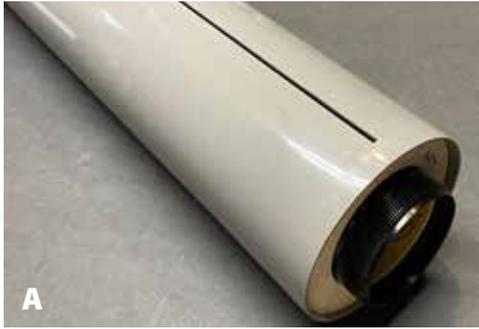
**A. Dry fit** (NO EPOXY!) the motor tube/centering ring assembly into the airframe.
