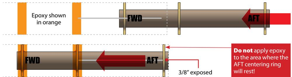
**DO NOT APPLY EPOXY WHERE THE AFT CENTERING RING WILL REST!!!** You will need to slip the AFT centering ring off the motor tube in a future step. Push the motor tube assembly into the airframe.
