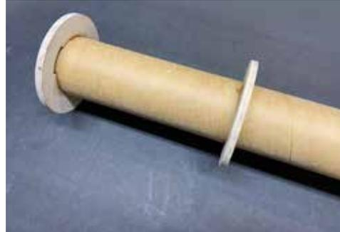
**B.** Dry fit all centering rings into the airframe and over the motor mount tube. The FWD notched ring and MID standard ring can be a little snug in the airframe and on the motor tube. If it is too tight, sand the ID and/or OD for a better fit.
