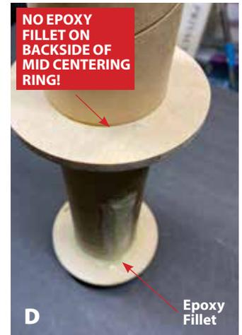
**NO EPOXY FILLET ON BACKSIDE OF MID CENTERING RING!**
