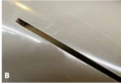
**B.** Make sure the MID and AFT centering rings do not interfere with the fin slots.
