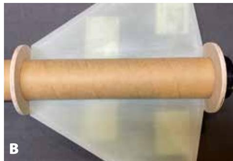
**B.** **Dry fit** the fins between the AFT centering ring and the MID centering ring. This gives you an accurate location of where the mid centering ring should be placed. Using cyanoacrylate glue (super glue), lightly tack the MID centering ring in place.
