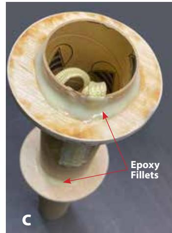
**C.** Make an epoxy fillet on the topside of the FWD notched centering ring and the MID centering ring.
