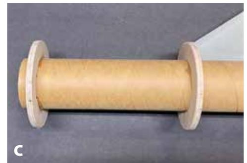
**C.** Locate the FWD notched centering ring 1/2" from the FWD end of the motor tube. Tack in place using cyanoacrylate glue.
