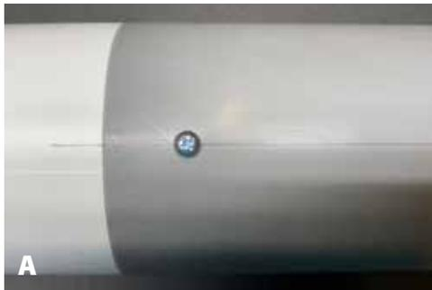
**A.** Slip the nosecone into the top of the payload section tube. Secure the nosecone to the payload section with 3 small screws or removable plastic rivets equally spaced around the circumference of the payload section tube about 1" below the nosecone. Be sure to pre-drill holes of the appropriate size when using screws. 1/4" long sheet metal screws work well in this application. If you prefer to use PML Removable Plastic Rivets (RVT-24), you will need to drill 5/32" diameter holes.
