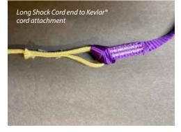
payload bay bulkhead. Most builders use a quick link (not included) for this purpose. A quick link makes it easy to change out shock cords if needed.
