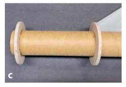
**C**. Locate the FWD notched centering ring 1/2" from the FWD end of the motor tube. Tack in place using cyanoacrylate glue.
