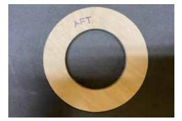
**C**. Use a pencil to mark the AFT centering ring for identification. *You do not want to switch the MID and AFT centering rings during assembly!* The AFT standard centering ring should be looser in the airframe and over the motor mount tube; you will need to slip the AFT centering off the motor tube while it is in the airframe during a later step. Sand the ID and/or OD for a loose fit if necessary.
