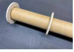
**B**. Dry fit all centering rings into the airframe and over the motor mount tube. The FWD notched ring and MID standard ring can be a little snug in the airframe and on the motor tube. If it is too tight, sand the ID and/ or OD for a better fit.
