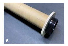
**A**. Slip the MID then AFT centering ring over the motor tube. Then **dry fit** (NO EPOXY!) the motor retention ring onto the motor tube. Make sure the retention ring is all the way onto the motor tube (approx. 3/8"). Slip the AFT ring down so it butts up against the retention ring
