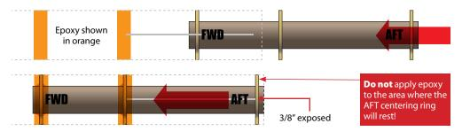
**DO NOT APPLY EPOXY WHERE THE AFT CENTERING RING WILL REST!!!** You will need to slip the AFT centering ring off the motor tube in a future step. Push the motor tube assembly into the airframe.
