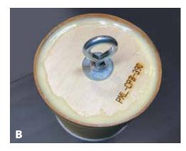
**B**. Spread a layer of epoxy around the inside circumference of the coupler to a depth of about 1/2".
