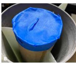
D. Remove the tape tabs from the centering ring and permanently epoxy it in the base of the rocket. *The motor tube must protrude*3/8" from the face of the centering ring!
