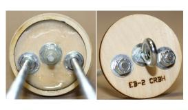
STEP 4 Place other bulkhead onto end of coupler. Use a long stick and epoxy fillet the intersection where the stepped bulkhead meets the ID of the coupler. Allow to cure.
