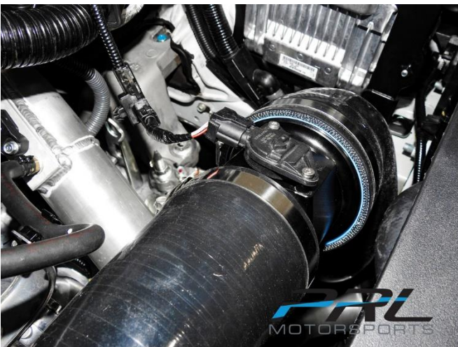
25. Loosely attach the large side of the billet MAF sensor housing to the 4" silicone hose and finish attaching the connected upper housing assembly to the factory black plastic inlet pipe.
