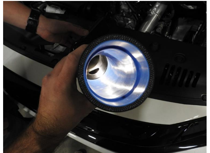
24. Loosely attach the upper intake hose to the billet MAF sensor housing, making sure the radius of the hose angled up and that the MAF housing is butted up against the hose's pocketed receiving groove for smooth airflow.
