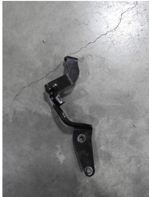
15. Remove the two 10mm bolts that attach the lower air box bracket to the chassis
