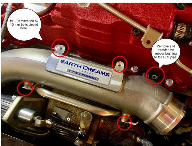
4: Remove the two 10mm bolts holding the wire harness shown in red circles. Remove the two 14mm bolts shown in white circles that attaches the inlet housing to the compressor side. Unplug the wire harness for easier access to one of the 14mm bolts. An extension will be needed for this, preferably with a swivel head. Various lines may need gently held out of the way to access all of the bolts.
