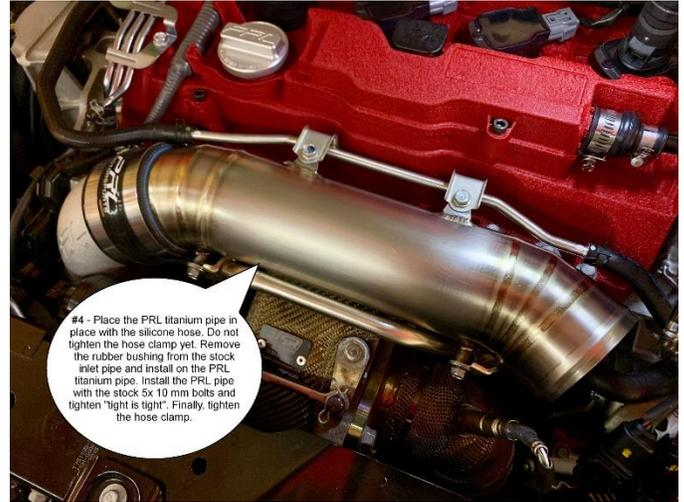
7. Reinstall the connection to either the factor airbox or the stock airbox. Tighten the casting side of the inlet pipe silicone clamp.
