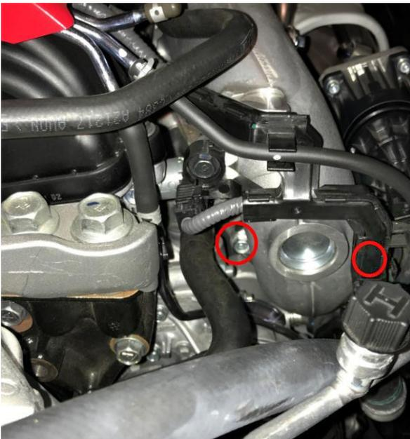
5: Install the PRL cast aluminum inlet section by reusing the two 14mm bolts that connect to the compressor inlet along with the stock black metal gasket. Note orientation of the stock gasket on the stock piece. Reinstall two 10mm bolts for the wire harness. Re-install the wire harness and install the PRL silicone adapter with the hose clamp on the casting side. Make sure to push the coupler fully on until it meets the stopper inside.
