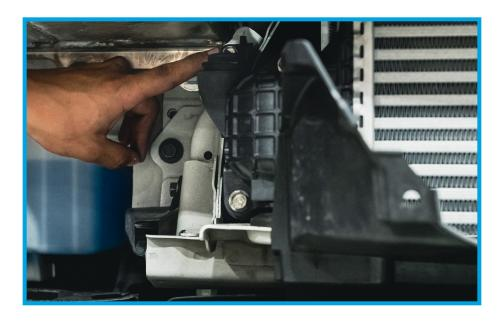
7. Remove the (2) factory 10mm bolts per side of the factory intercooler. Make sure to keep these bolts, as they will be reused with the PRL Intercooler.
