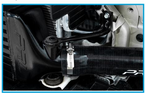
18. If you have not already done so, torque down the (2) factory 12mm bolts on passenger side of the end tank to the factory charge pipe.
