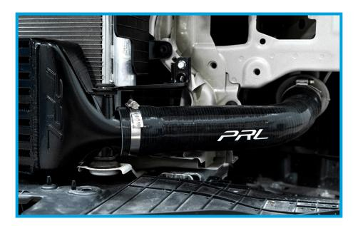
20. Before you reinstall the now trimmed bumper beam, you will need to trim the plastic air guide to fit correctly. There should be an air gap all around the PRL Intercooler, the bumper beam should not make contact with it at all.
