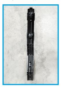
10. The bumper beam needs to be trimmed to provide clearance, as the PRL intercooler is far larger than factory. You will need to remove the (5) 14mm & (1) 10mm factory bolts, per side to remove the bumper beam.
