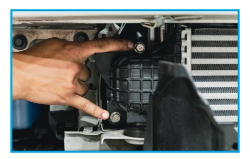
8. Remove the (2) rubber grommets from the factory intercooler and place them on the PRL Intercooler. This will let the intercooler sit in the mounts.
