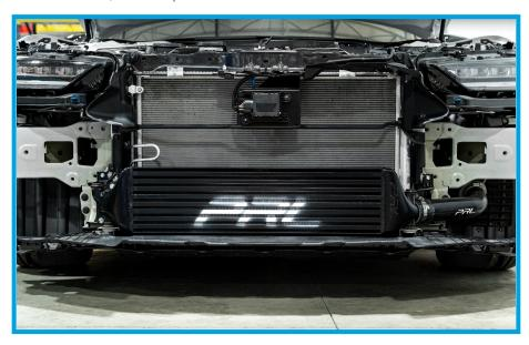
21. Once the bumper beam is re-installed, follow the bumper removal steps in reverse, making sure to re-install all harnesses.
