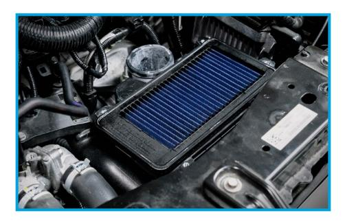
10. Place the PRL Stage Silicone Hose on the factory inlet and airbox. Tighten the (2) worm gear clamps. Reclip the MAF sensor into its housing.
