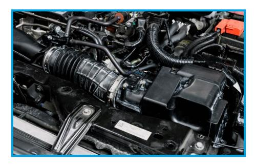
6. Pinch the back of the MAF sensor clip firmly and pull straight away from the MAF sensor housing. Be sure to not damage the sensor. Tuck out of the way.
