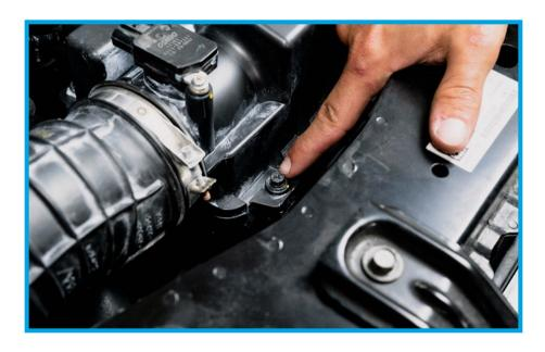
8. Remove the (2) factory clamps holding the corrugated hose to the airbox. This hose and clamps will not be re-used.
