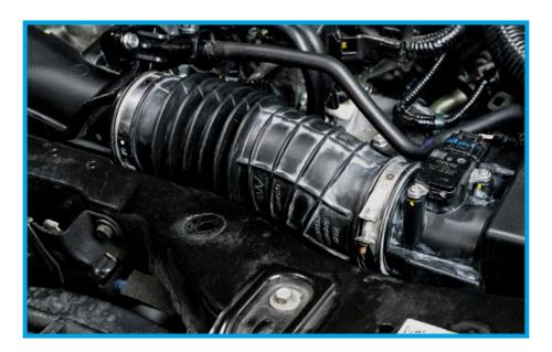
9. With the lid of the factory airbox off, remove the factory filter and replace with the PRL Panel Air Filter. Re-seal the factory airbox.
