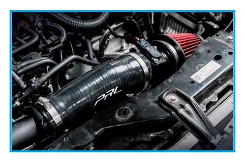
14. Re-clip the MAF sensor harness into place. Ensure that all clamps are tightened fully.
