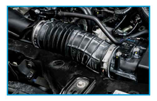
8. Remove the (2) Phillips head screws that holds the MAF sensor into the factory MAF housing. These screws will not be re-used.
