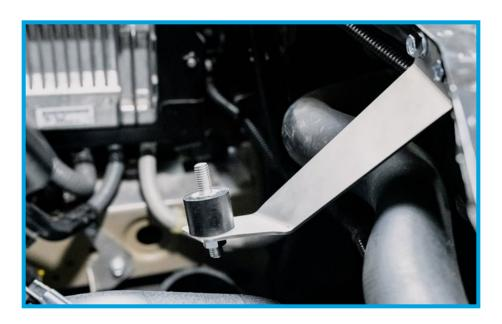
12. Seat the MAF housing with the onto the Rubber Vibration Damper so that it stays in the correct position.
