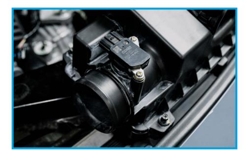
9. Remove the MAF sensor fully from the factory airbox and place it into the PRL MAF housing. Using the supplied (2) M4 bolts and secure the sensor into place.
