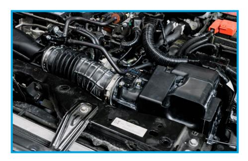
6. Pinch the back of the MAF sensor clip firmly and pull straight away from the MAF sensor housing. Be sure to not damage the sensor. Tuck it out of the way.
