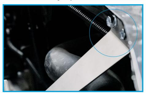
11. Insert the M8 Rubber Vibration Damper and tighten the Serrated Flange nut to the underside of the grommet to lock it in place
