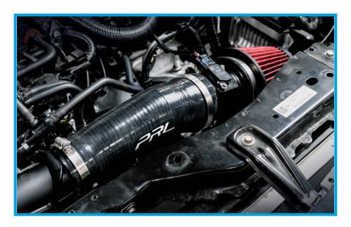
14. Re-clip the MAF sensor harness into place. Ensure that all clamps are tightened fully. The vehicle will then require an ECU calibration for the MAF.
