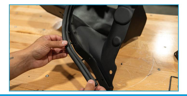
Install the rear rubber bushing and sleeve from the OEM air box into rear pocket of the PRL air box. Install rubber bushing from bottom of OEM air box into the bottom of the PRL air box.
