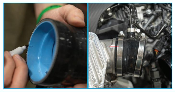
Place the other silicone coupler labeled SIL-FL5-INT-HVI-HOSE-B and (2) worm clamps on the MAF housing that you connected to the airbox. The hose clamp on the MAF housing side will be the larger of the remaining hose clamps. Place one of the smaller hose clamps #9 on each open end of the 2 silicone connectors.
