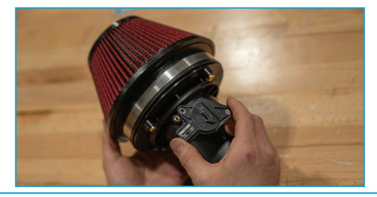
Attach HVI MAF housing to the HVI intake air box using provided M5x12 flat head cap screws and dress up washers. Torque them to 15 in-lbs.
