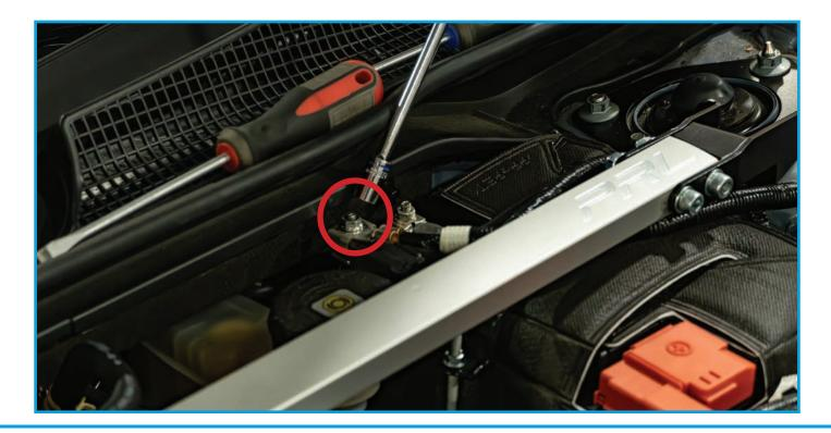
Loosen the 4 hose clamps on factory OE rubber connectors. Remove the valve cover vent hose from rubber boot connecting to OEM inlet pipe. Remove both the rubber connecting boots but leave plastic EVAP Purge Jet housing in the car.
