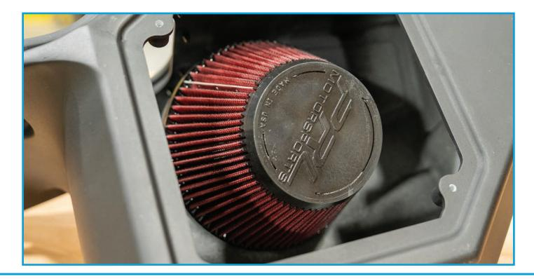
Install air box side panel using the (4) included M5x10 flanged button head cap screws. #18. Set the entire assembly aside for now.
