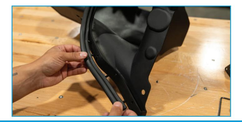
Install Rear rubber bushing and sleeve from OEM air box into rear pocket of the PRL airbox. Install rubber bushing from bottom of OEM airbox into the bottom of the PRL airbox.
