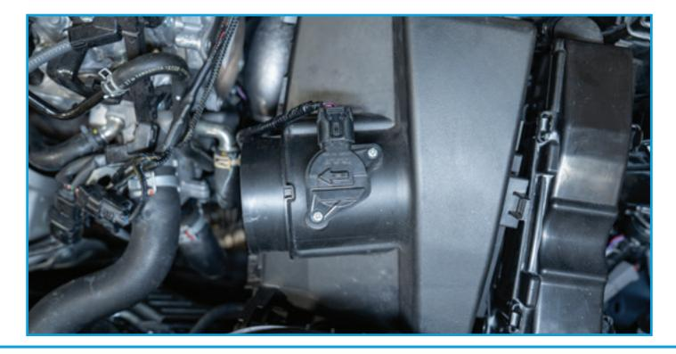
Remove the airbox bolts holding the airbox in the engine bay. 1 on back side, one on right side and 2 in front on airbox scoop. Pull the airbox from the engine and side aside.
