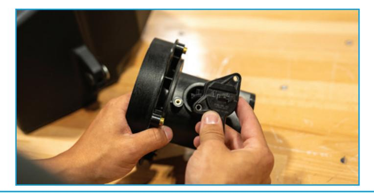
Attach HVI MAF housing to the HVI intake airbox using provided M5 x 12 flat head cap screws and dress up washers. Torque to 30 in-lbs.
