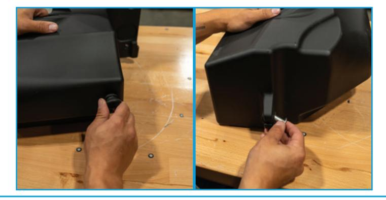
Place the included worm clamp on to the the new filter and install onto provided PRL Maf Housing. Tighten worm gear clamp to 30 in. lbs.
