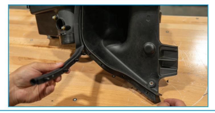
Install weather stripping to PRL HVI. Make sure to align the clips in the correct orientation. it will only fit correctly one way.
