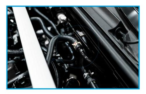
9. Using a pair of pliers, squeeze the tension clip to loosen the line. Then you can rotate the hose freely to provide ample gap underneath the strut bar.
