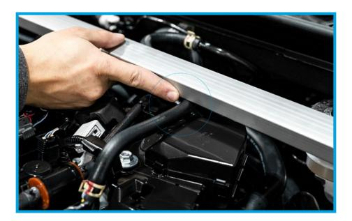
8. If the line is touching, you will have to adjust the rotation of the EVAP line. There is a tension clip that will have to be loosened for the line to rotate.
