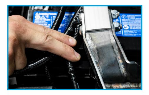
7. Ensure that there is clearance of the EVAP line on the right side of the motor. The line should not make contact with the bar itself.
