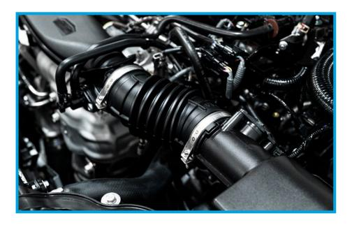
7. Place the (2) provided worm gear clamps onto each end of the silicone and tighten with a Philips head screwdriver.
