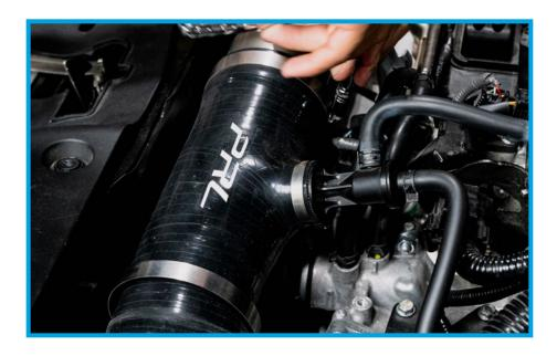
32. Attach the (2) PRL vacuum hoses to the PRL EVAP assembly and reinstall them reusing the factory hose clamps. Couple to your specific PRL MAF & intake.
