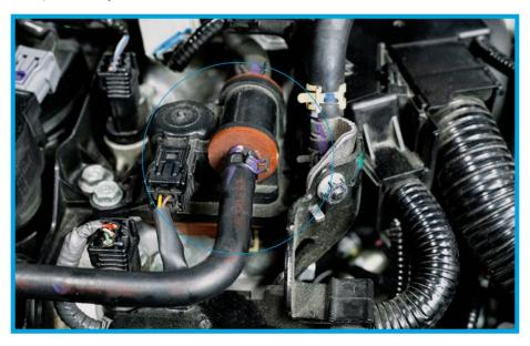
PLEASE NOTE: The below vacuum line is not present and is not used on INTERNATIONAL MODELS ONLY. A cap for the EVAP Assembly is provided.
