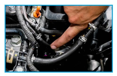
27. Attach the wastegate harness to PRL Compressor inlet using provided fir tree zip tie. Reconnect wastegate harness. Push firmly, as plug may "clip" but not make a full connection. This will give an error code on startup.
