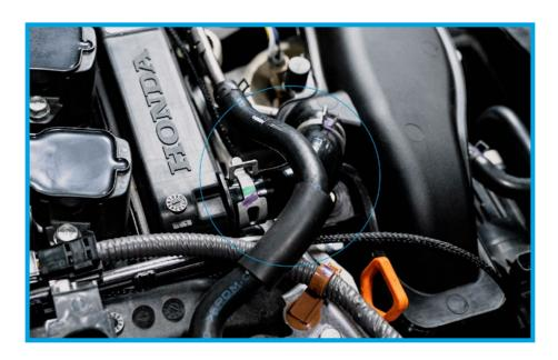
9. Disconnect the compressor outlet hose. Loosen the (1) factory worm clamp with a Phillips head screwdriver. Tuck the hose out of the way towards the fender.
