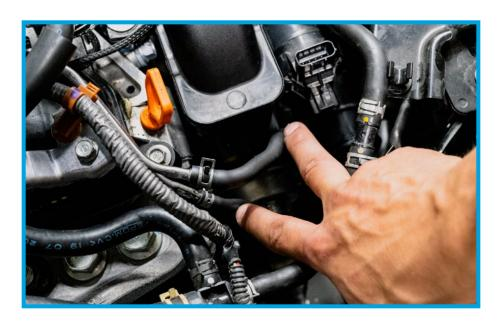
16. Remove (1) 12mm bolt in the factory inlet located under valve cover breather hose location. This factory bolt is reused for the PRL Turbo Inlet.
