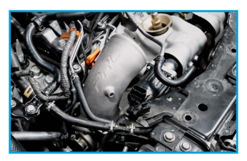
25. Re-attach compressor outlet hose to the PRL Compressor outlet nipple. Use Phillips head to tighten factory worm clamp.
