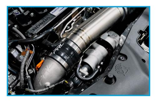
34. Ensure the wastegate harness, EVAP Assembly, MAF sensor and vacuum lines are all secure. Reinstall plastic shroud using the factory clips.
