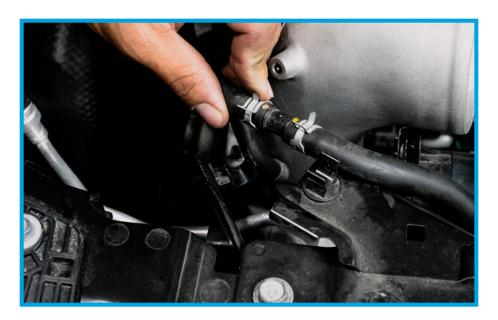
29. Seat the smaller silicone on the inlet, affix the breather connection with the small #10 worm clamp. Tighten the (1) #48 worm clamp on the compressor inlet.
