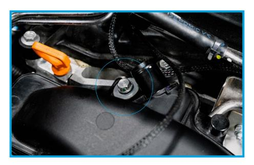
17. Remove (1) 12mm bolt located next to the EVAP assembly. This factory bolt, mounting grommet and washer will be reused with the PRL Inlet Pipe.
