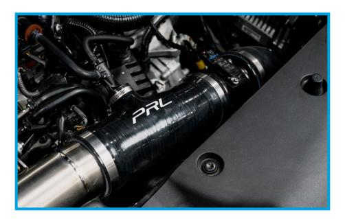
33. Align the Titanium Inlet & Upper Intake Silicone as needed for smoothest airflow, then tighten (3) #48 worm clamps and grommeted mounting bracket.
