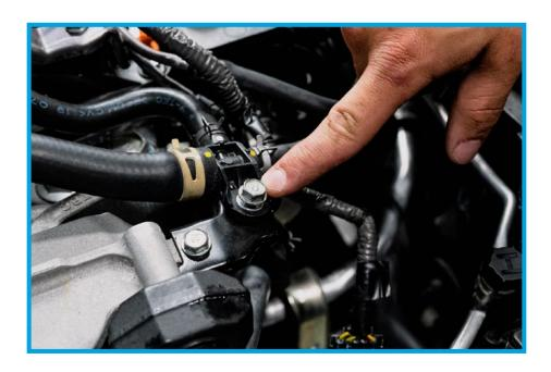
15. Remove (2) factory vacuum lines. Reuse (4) factory clamps on the provided PRL vacuum lines. Use pliers to squeeze the clamps to easily remove them.
