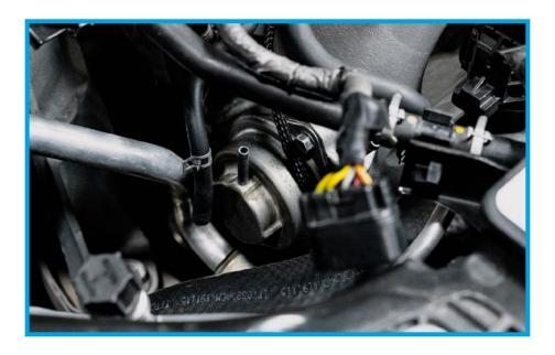
22. Transfer the mounting grommet into the PRL Titanium Inlet Pipe. It's advised to wear gloves during this step. Clean surface if any fingerprints/marks are left.
