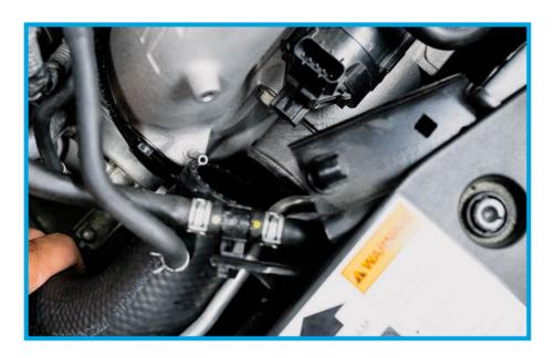
26. Install (2) PRL Vacuum lines, reusing the factory clamps. Use pliers to squeeze the clamps to easily place them into their position.
