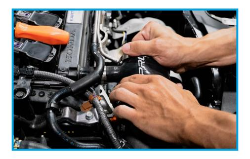
30. Insert Titanium Inlet gently and loosely attach to factory mounting point reusing the factory grommet, washer & bolt. Do not tighten down yet.
