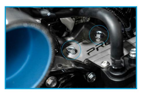
37. Remove this small bracket from the the blue factory clip that holds it on the harness. It is not necessary and should be removed.
