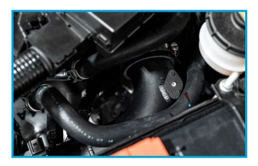
34. Replace the factory heater hose bracket into the PRL hardpipe using (1) of the provided M6 Flange Bolts. Do not clip the hoses back into place until the end.
