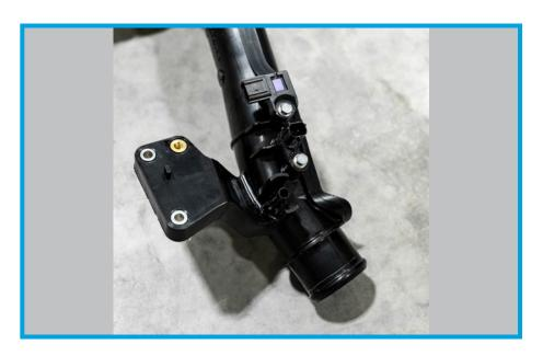
31. Install the MAP sensor and IAT sensor with the (1) 10mm factory bolt into the hardpipe. The 1/4" Hose Barb to 4an comes pre-installed in the last hole in the hardpipe.
