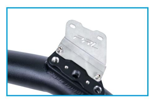
36. Bolt the PRL hardpipe to it's mounting points using the (2) remaining M6 Flange Bolts provided.
