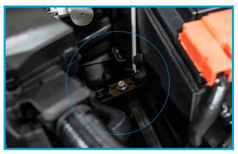
21. Remove the (2) 10mm factory bolts from the bracket that holds the factory hardpipe to the engine block. Remove the (1) 10mm factory bolt holding the small bracket that is clipped to the harness. These factory bolts are not reused.
