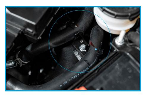
42. Fit the PRL Stock Intercooler Charge Pipe Adapter into the lower side silicone. Make sure the o-rings are properly seated. Bolt the charge pipes to either the factory intercooler or the PRL Intercooler using the (2) factory bolts.
