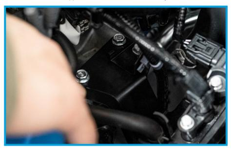
22. Remove the MAP sensor and IAT sensor from the factory hardpipe. These are both clipped into the factory hardpipe, be careful to not damage them.
