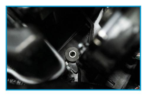
17. With all hardware loosed and removed, wiggle the airbox free of the solid post it is seated on in the engine bay. Be careful to not bend or snap it off.
