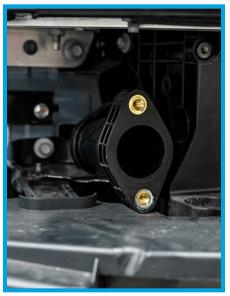
27. Using a Philips head, loosen the factory hose clamp on the hot side hose attached to the turbo. This clamp and hose will not be re-used.
