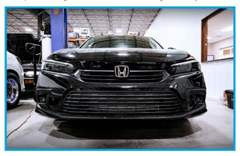
5. Remove the (3) bumper clips above each headlight. You can utilize a flathead screwdriver, or a clip removal tool. Be sure to not damage the clips during this process. If any are snapped, visit your local Honda dealer for replacements.
