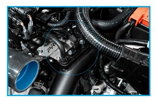
41. Clip the heater hoses into place in the factory bracket that is mounted into the PRL hardpipe.
