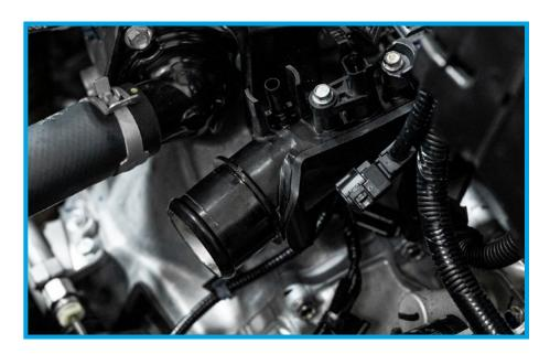
26. Remove the (2) 10mm factory bolts from each of the factory charge pipe connections to remove them from the intercooler. If you are also installing a PRL Intercooler, this is where you would begin installation for the intercooler. For full PRL Intercooler installation guidance, refer to the PRL Intercooler Install Guide.
