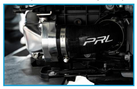
43. If you have PRL High Volume Intecooler Outlet, you WILL NOT use the intercooler adapter. You will place the Intercooler Outlet directly into the lower cold side silicone.
