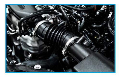
15. You will need to remove the (2) 10mm factory bolts that hold the air duct to the factory airbox.
