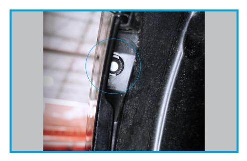
9. On the underside remove (10) bumper clips along the front section. They are circled in blue in the image below. There are (1) 10mm shoulder bolts and (1) Phillips head screws per side. They are circled in white in the image below.
