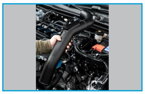
32. Install the PRL Throttle Body Silicone Coupler to the throttle body. Tighten the (1) IFE 60-80-12 hose clamp on the coupler, affixing it to the throttle body.
