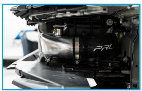
44. If you are installing the PRL Intercooler, you will also have to flip the ambient air temperature sensor to face outward, as it will not clear with the PRL intercooler installed. This isn't necessary with the factory intercooler.
