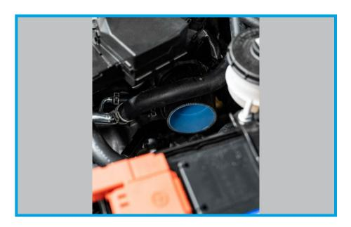
33. Work the PRL hardpipe into positon and it is angled correctly out of the throttle body and tighten down the other clamp down.
