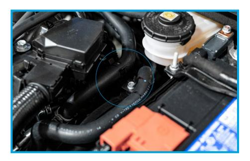
19. Remove the (1) flat head screw that holds the factory charge pipe to the throttle body.
