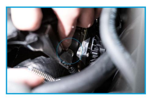
20. Remove the (1) 10mm factory bolt from the factory bracket the holds the heater hose. This bracket is reused, the factory bolt is not.
