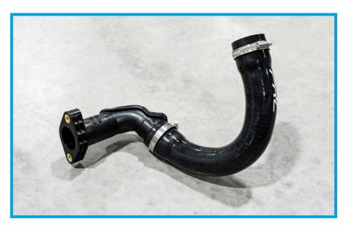
29. Tighten down the connector side clamp, and then install the hot side PRL Silicone onto the turbo. Tighten down the other clamp fully at this time.
