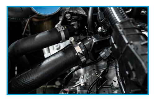
25. Pull the factory hose from the bottom of the factory hardpipe. You will then need to fully disconnect it from the intercooler to fully remove this hose.
