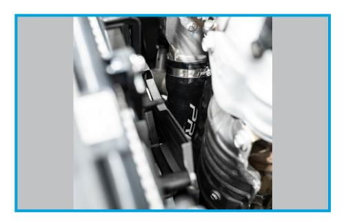
30. Remove the MAP sensor and the IAT sensor from the factory hardpipe. There is (8) 10mm factory bolt holding each into place in the hardpipe.
