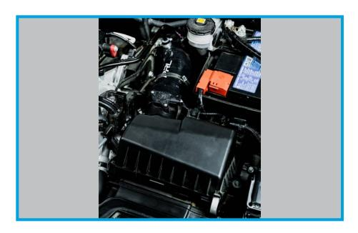
12. Tighten all (3) provided hose clamps with a flathead screwdriver. Be careful to no overtighten, as you could create gaps or deform the factory airbox outlet. Check to make sure all connections are secure.
