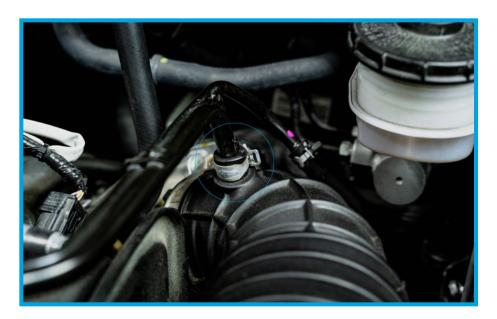
7. Free the EVAP lines from the factory hose, and loosen and remove the factory hose off the engine and factory airbox. Remove from the engine bay.
