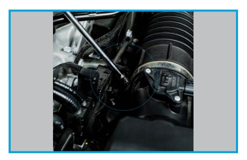
5. Using a 12" extension with a 5.5mm socket, loosen the second factory hose clamp holding the factory hose to the throttle body.
