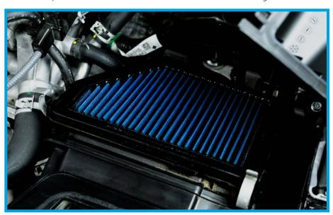
11. Close and secure the lid with the clip, re-attach the MAF sensor harness clip and affix the silicone to the factory airbox.
