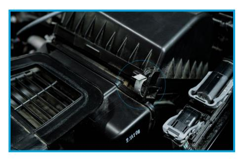
9. Place the PRL silicone with clamps equipped into the engine bay. Affix the throttle body side first, insert the EVAP line into the top bung, but do not tighten down the hose clamps yet. This will allow you to adjust fitment.
