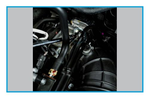
6. Using needlenose pliers, remove the tension clip that holds the factory EVAP lines to the factory hose. This clamp will not be re-used.
