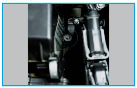
13. With the bolts removed, wiggle the airbox side-to-side, while pulling upwards. This will free it from the engine bay mounting post.
