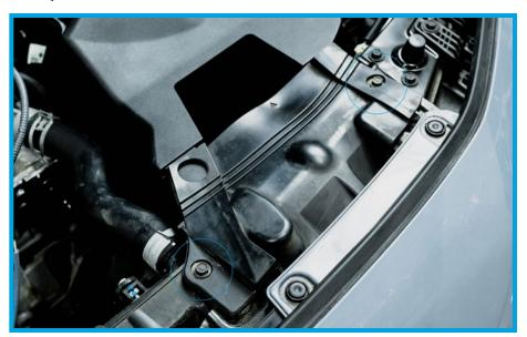
35. Once the duct is re-attached, check all connections to ensure everything is tightened and secured in the correct position. Clean a flat visible surface under the hood and affix the enclosed CARB EO Sticker for SMOG purposes. (CALIFORNIA VEHICLES ONLY)
