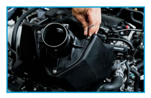
19. Using (2) of the provided flanged button head screws, affix the PRL Mounting bracket to the side of the PRL High Volume Airbox. Keep loose for desired fitment adjustment. Tighten once fitment is as desired.
