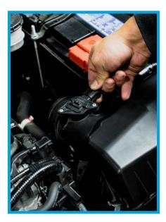
5. Unclip the MAF sensor harness from the factory airbox lid using a set of needlenose pliers. Squeeze the tab to free it from the lid's mounting point.
