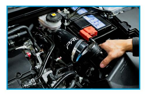
25. Affix the other end of the silicone hose onto the PRL High Volume Airbox. You will have to use an even, firm amount of pressure to do this.
