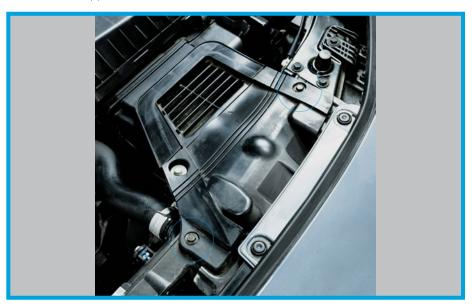
7. Using a 12" extension with a 5.5mm socket loosen the first factory hose clamp holding the factory hose to the factory airbox.
