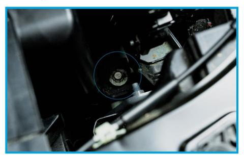
12. Using the 12" extension, remove the factory 10mm bolt located on the right side and near the rear of the factory airbox. This bolt will be NOT re-used for the PRL HVI Airbox.
