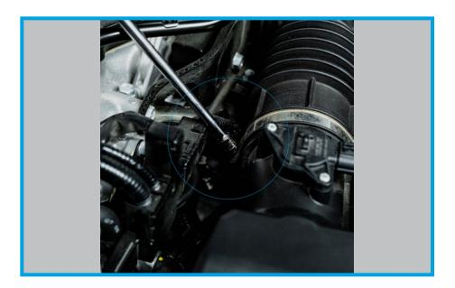
8. Using a 12" extension with a 5.5mm socket, loosen the second factory hose clamp holding the factory hose to the throttle body.
