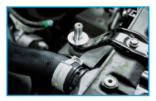
17. Place the PRL High Volume MAF Housing with the filter attached into the airbox. It's easier to mount this with the airbox still out of the engine bay.
