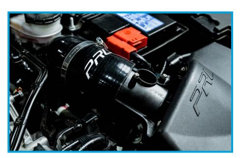
26. Seat the PRL High Volume Airbox onto the (2) mounting posts. You will need to press down firmly once you know they are lined up.
