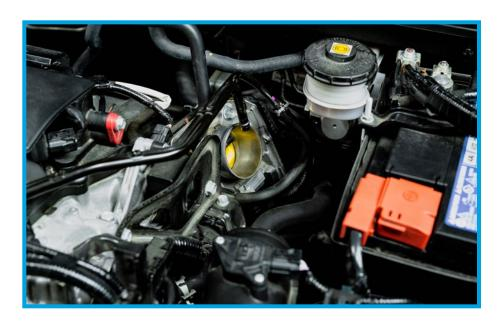
11. Using a 12" extension, remove the factory 10mm bolt located on the right side and near the front of the factory airbox. This bolt will be re-used for the PRL HVI Airbox.
