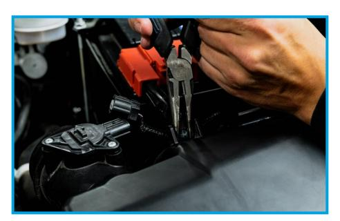
6. Remove the (2) factory 10mm bolts that hold the factory intake duct from the core support. These bolts will be re-used to affix the rubber ducting back to the core support and it will be affixed to the PRL HVI Airbox.
