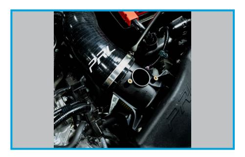
29. If you have not already, push the EVAP lines into the top bung of the PRL silicone. Using a flathead screwdriver, tighten this smaller hose clamp.
