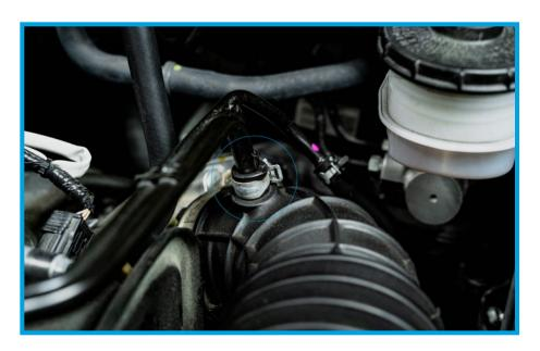
10. Free the EVAP lines from the factory hose, and loosen and remove the factory hose off the engine and factory airbox.
