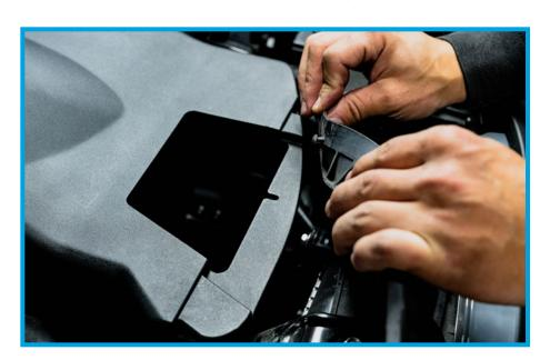
34. Secure the factory rubber ducting back to the core support with the (2) factory 10mm bolts.
