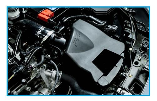
27. Using the (1) factory 10mm bolt, thread it through the grommet and fasten the front of PRL High Volume Airbox down in the engine bay.
