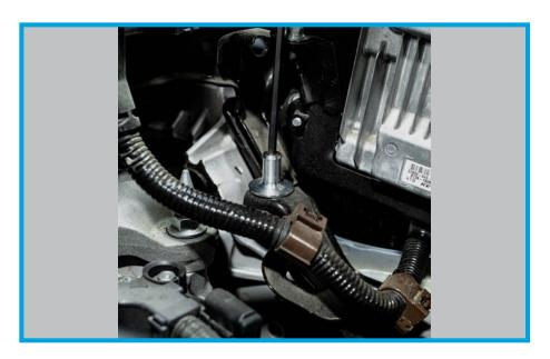
16. Secure the remaining PRL Mounting post to the bracket on the core support with the remaing M6 socket head screw This is tightened using a 5mm Allen wrench.
