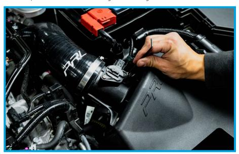
32. Clip the MAF sensor harness into the MAF sensor itself. There should be a slight click when it is secured into place.
