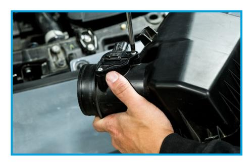
31. Place the MAF sensor into the PRL High Volume MAF housing. Using the (2) M4 socket head screws affix the MAF sensor in place. This is sec Be sure to not over-torque these screws. This is tightened using a 3mm Allen wrench.
