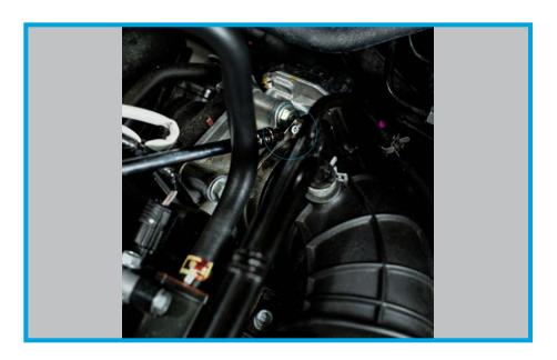
9. Using needlenose pliers, remove the tension clip that holds the factory EVAP lines to the factory hose. This clamp will not be re-used.
