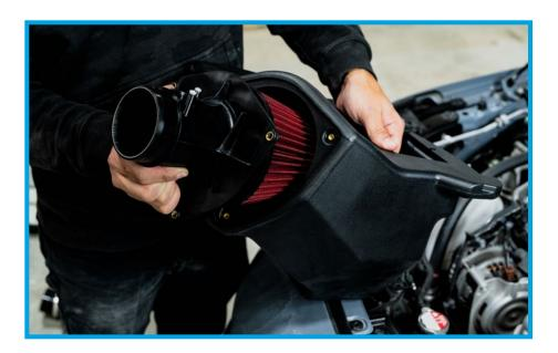
18. Using (3) of the provided flanged button head screws, affix the MAF Housing to the PRL High Volume Airbox. This is tightened using a 3mm Allen wrench.
