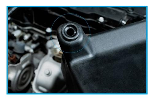
21. Using the remaining provided PRL Rubber Grommets, place it firmly into the opposite hole in the bottom of the PRL High Volume Airbox.
