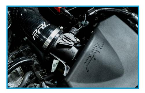
33. Take the factory rubber ducting and secure the nipple located on the bottom of it into the slot on the top of the PRL High Volume Intake Airbox.
