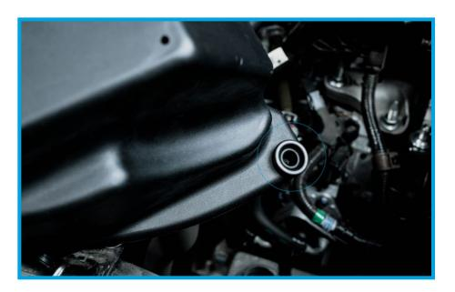
22. Remove the factory grommet out of the corner of the factory airbox. Pulling firmly to the side will allow it to come free of the factory airbox.
