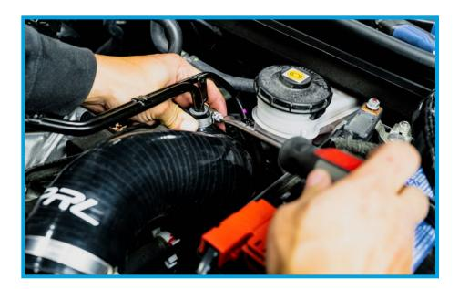
30. Using a Phillips head screwdriver, carefully remove the MAF sensor from the factory airbox. These screws will not be used in the PRL High Volume Intake Airbox.
