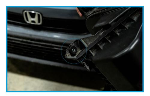
23. Place the factory grommet in the mounting bracket that is affixed onto the PRL High Volume Airbox. Pushing firmly, it will slide into the side of the bracket.
