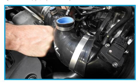
29. Place the small vacuum nipple into the silicone inlet hose. Slowly work the turbocharger inlet side of the silicone inlet hose onto the inlet pipe by pulling on the silicone. Slide the #44 worm clamp onto the silicone inlet hose.
