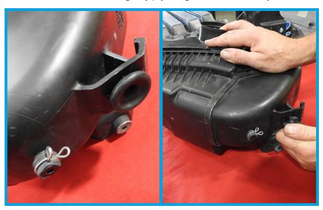
21. Re-install the rubber locator grommet on the bottom of the PRL HVI Air Box the same as it was removed from the stock air box. Lubricant can be used if necessary. If so, be sure to clean and dry up any excess.
