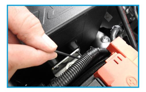
35. Attach the factory rubber air duct seal to the PRL HVI Air Box by pressing the clips into the slots. Start at one end, working towards the other making sure not to miss any connections, and that it is even and flush.
