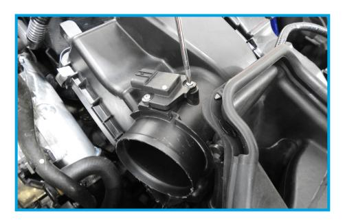
11. Carefully place the MAF sensor off to the side in a dry and clean location.
