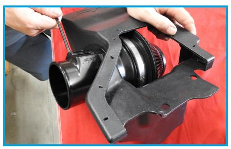
5. Loosely attach the HVI Air Box lid with (8) M5x10mm flange bolts. Work from one side of the box to the other, then when all bolts are placed and set, secure TIGHTLY using the long end of Allen wrench to ensure proper torque. Make sure bolts are tight, but be careful to not splinter the plastic of the HVI Air Box lid.
