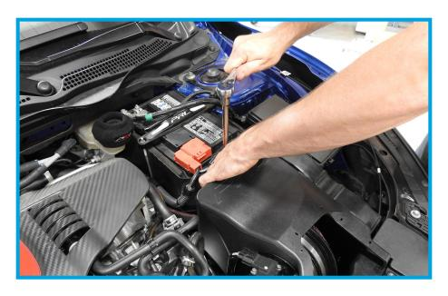
33. Using the (2) Flush Dress-Up Hardware Bolts to replace the stock 10mm bolts, tighten them down to affix the front of the HVI Air Box. You can also utilize the factory shoulder bolts, if you would prefer.
