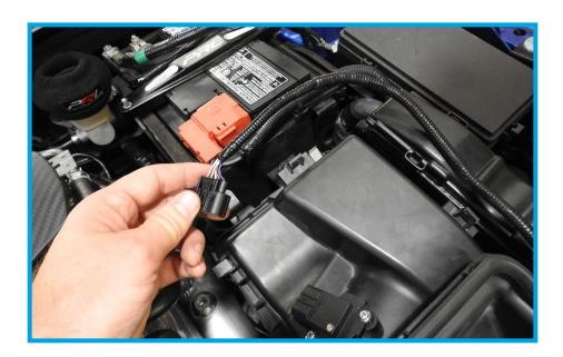
10. Remove the MAF sensor from the factory MAF housing with a Phillip's head.
