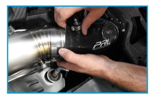
30. Place the PRL EVAP Assembly (Ver. 2) into the silicone inlet hose. Attach the factory EVAP purge valve to the PRL EVAP Assembly. Intakes purchased before 2021 may have Version 1 of the EVAP assembly. Installation will vary slightly for that EVAP Assembly. Please contact support with any questions.
