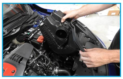
18. Remove the rubber mount on the back of the factory air box by pressing down to slide the metal sleeve located in the middle. The rubber grommet will then be able to be pressed out. This requires a little bit of force.
