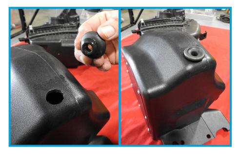
22. Install the MAF sensor into the PRL Billet MAF Housing using the (2) M4x8mm socket head cap screw bolts.
