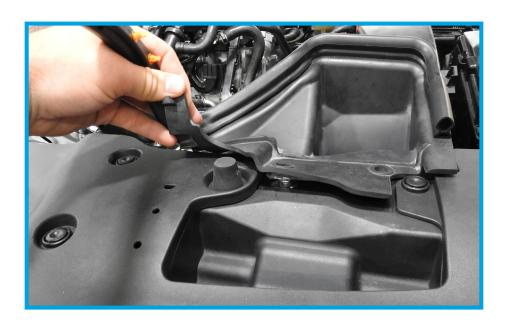
17. Lift on the stock air box to remove the assembly from the engine bay. This may require a slight back and forth motion to release it from the rubber locator.
