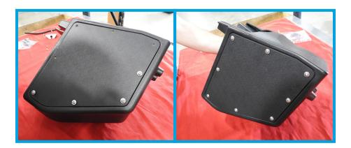
6. Attach the supplied air box bracket using the remaining (2) M5x10mm bolts.
