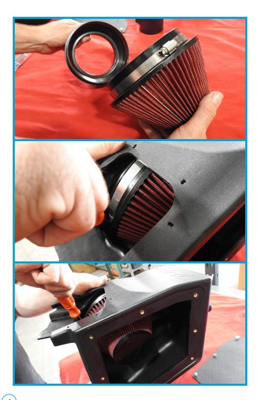
4. Attach the Mass Air Flow Sensor (MAF) housing to the PRL Velocity Stack by aligning the holes through the HVI Air Box with the (4) M6x16mm socket head screw bolts. \*TIGHTEN USING THE LONG END OF ALLEN WRENCH FOR TORQUE\*
