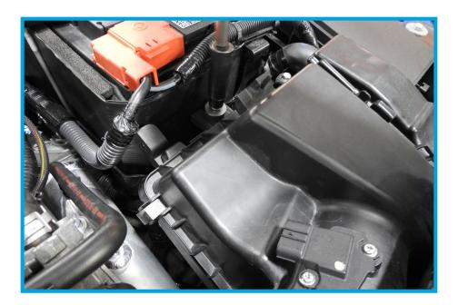
14. Remove the (1) 10mm bolt located between the ECU and the stock air box. At least a 12" extension will be needed to reach this bolt, it's a narrow space and located on the lower section of the engine bay.
