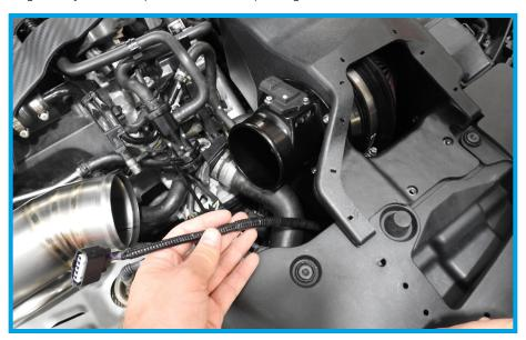
25. Place the PRL HVI Air Box into the engine bay. Make sure to line up the bolt holes and align the lower locating grommet into place. Press down firmly to push the lower locating grommet into place.
