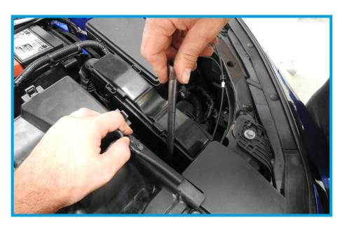
15. Remove the air duct seal by releasing the plastic tabs. Typically this can be removed by pulling towards the left side of the detent tabs. A flathead screwdriver may be needed for leverage if this is problematic to release. Be careful to not tug or stretch on the air duct seal rubber.
