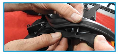
16. Lift up on the rubber tab on the air box seal using a flathead screwdriver. Make sure not to pry too hard to snap or crack the plastic.
