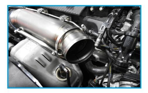
28. With the HVI Air Box still loosely installed and unbolted, attach the silicone inlet hose to the billet PRL MAF housing with the #52 worm clamp. Do not tighten the clamp yet, adjustments may need to be made for fitment sake.
