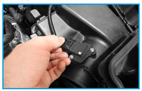
9. Remove the MAF sensor wiring harness from the retaining clips and casing by using a flathead screwdriver to release the detents. Carefully pull this harness and the exposed wiring to the side out of the way.
