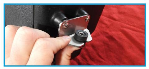
20. Remove the rubber locator grommet on the bottom of the stock air box. Use a flathead screwdriver to gently pry this grommet if necessary.
