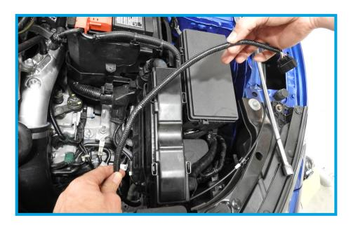
24. Route the MAF sensor wiring harness down towards the center of the engine bay as far as possible without putting tension on the harness.
