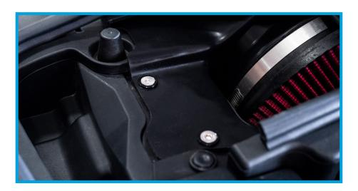
34. Using the long end of Allen wrench to ensure proper torque, tighten down the (2) M5x10mm flange bolts connecting the rear bracket to the HVI Air Box.
