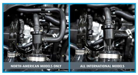
31. Rotate the PRL EVAP assembly as pictured to avoid part of the EVAP from rubbing the underside of the hood. If needed, you can slightly rotate the silicone inlet hose itself, and/or bend the hard lines out of the way for added clearance. Tighten the #8 and #20 worm clamps.
