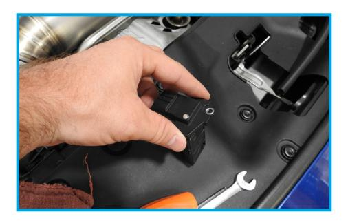
12. Remove the (2) 10mm bolts from the front of the air box.
