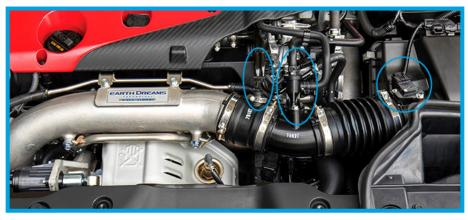
8. Disconnect the MAF sensor by pressing on the center of the clip and pulling outwards away from the mounted sensor bracket.
