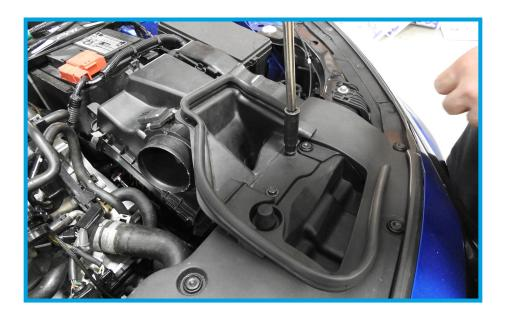
13. Remove the (1) 10mm bolt located on the back of the air box that goes through the rubber mount next to the battery.
