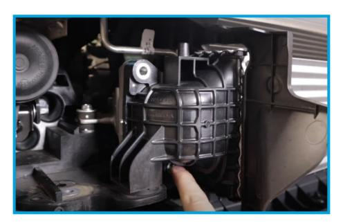
14. The intercooler is now loose, but not easily removed as the plastic covers and air guides holding the intercooler in place. Pull the bottom of the plastic towards you and the vertical guides to the side. Remove the factory intercooler.
