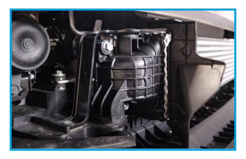
13. Remove the (2) bolts and bracket holding each side of the factory intercooler.
