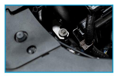
18. Push the (2) provided plastic rivets into place to affix the air duct and fully stabilize the airbox against the core support.
