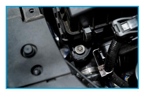
10. Wiggle the airbox free, pulling the airbox from the factory mounting post that is located on the back right side of the airbox.
