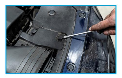
5. Once the clips are removed, you can remove the factory air intake duct entirely. These clips will not be re-used.
