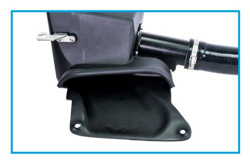
14. Put the provided rubber grommet into the bottom of the airbox. Seat the airbox onto the factory mounting post.
