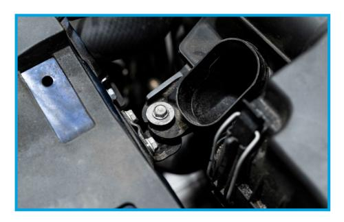
9. Remove the (1) factory 10mm bolt on the front right side of the factory airbox. This bolt will be reused in the PRL mounting bracket.
