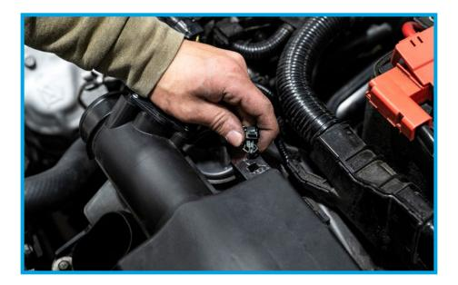
8. Remove the (1) factory 10mm bolt mounting the factory airbox to the core support. The bracket may be removed as well, as it is not utilized.
