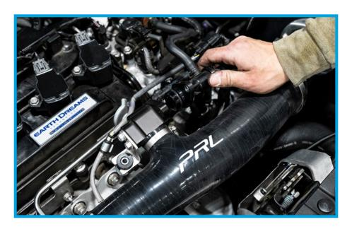
17. Replace the (1) factory 10mm bolt on the front right side of the airbox in the PRL Mounting bracket and factory rubber grommet.
