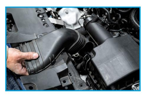
6. The factory corrugated intake hose will need to be removed. Loosen the (2) factory clamps to remove it from the factory airbox.
