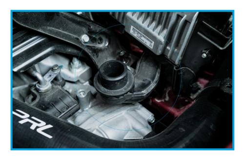
11. Before removing the resonator simply push back the (2) grey clips that lock the ECU into place. This will disconnect the ECU connections.
