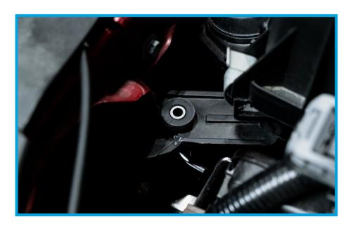
9. Remove the airbox by gently wiggling it free from the factory mounting post. It will expose the resonator under the factory airbox.
