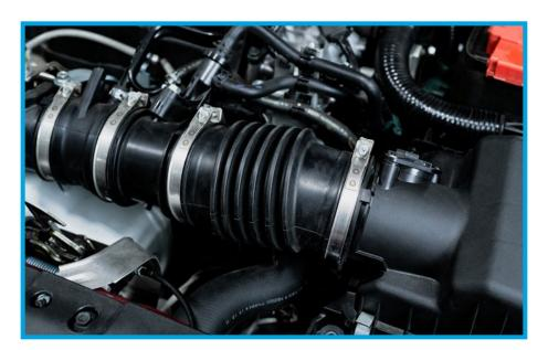
6. Unclip the MAF Sensor harness from the clip holding it into place and remove it from the MAF Sensor. Remove the MAF sensor from the factory airbox.
