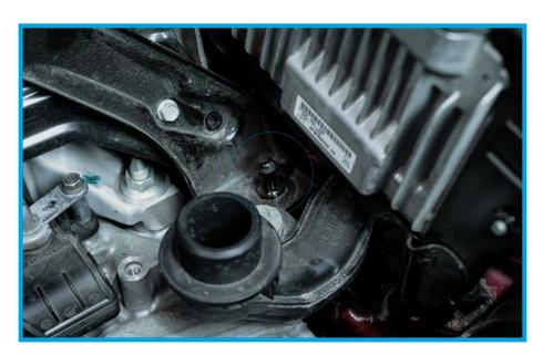
10. To fit the PRL High Volume Intake you will have to remove the factory resonator. This is under the ECU and the fuse box.
