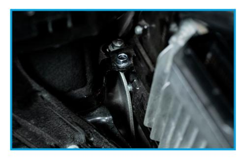
13. Remove the (1) factory 10mm bolt that is located in between the ECU and fuse box. This will allow the ECU to be lifted up out of the way.
