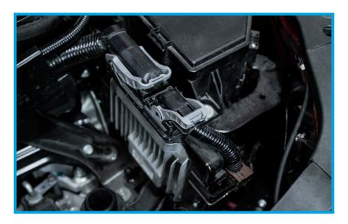
12. Remove the (1) factory 10mm bolt that is located behind the ECU, towards the battery. You will have to remove the lower bolt as well before removing.
