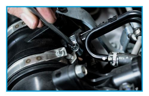
20. Using a pair of pliers, remove the tension clamps holding the EVAP lines to the factory EVAP assembly.
