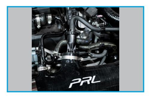
29. Push the (2) provided plastic rivets into place to affix the air duct, reconnect the MAF sensor harness and ensure all connections are tight and secure.
