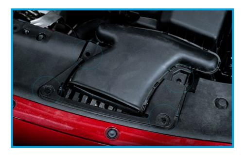
5. The factory corrugated intake hose will need to be removed. Loosen the (2) factory clamps to remove it from the factory airbox.
