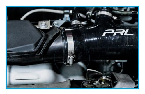
27. Place the MAF sensor into the PRL MAF housing and tighten it into place. Be careful to not over-tighten and damage the sensor.
