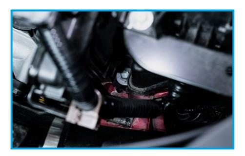
14. Remove the (2) factory 10mm bolts that hold the front of the resonator into place. These bolts and the bracket itself will not be re-used.
