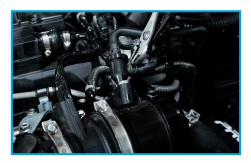
21. Remove the factory intake pipe from the inlet pipe and set aside. You will utilize all provided components to replace these connections.
