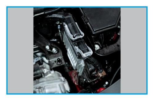
18. Loosen the (2) factory clamps on the factory intake pipe that connects to the factory inlet pipe. These clamps will not be re-used.
