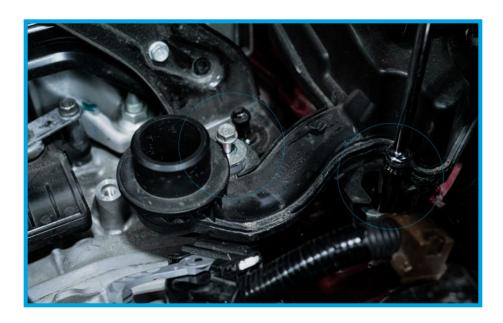
15. Free the back of the resonator by using a flat head screwdriver. Unseat the resonator off of the rubber grommet. Push inwards towards the engine.
