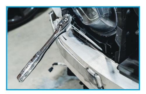
13. You can then access the bottom (2) bolts underneath the bottom plastic pan. Simply push down gently to access the bolts.
