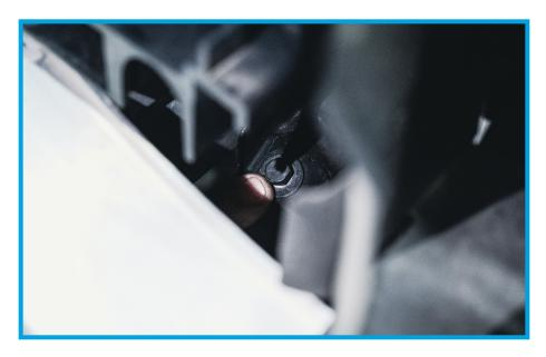
12. The bolt can be accessed via a 12" extension under the headlight.
