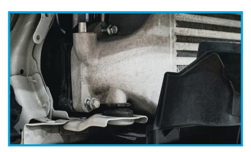
19. Replace Honda Sensing Unit back into position, torque hardware, reconnect the unit and then reconnect the front bumper by following the removal steps in reverse order. Replace any clips that may have been damaged during install with OEM Honda clips.
