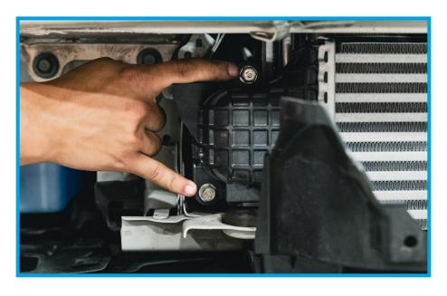
16. Loosen the factory clamp and push the hose away from the intercooler.
