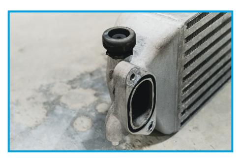
18. Torque down the (2) factory bolts on passenger side of the end tank. Use the suppled #40 Stainless Clamp on the driver's side.
