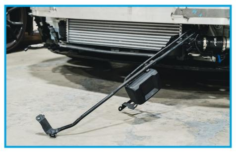
15. With the Sensing Unit removed, you will be able to access the sides of the factory intercooler to be able to loosen the (2) factory bolts holding it in place.
