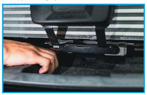
14. Simply pull the unit to the side and leave it propped up as to not put tension on any of the connections. If you have the car on jack-stands or a lift, fully disconnect the unit if it cannot be fully supported as pictured.
