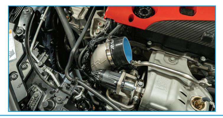
Install the new PRL Inlet Pipe into the elbow as shown below, aligning the rubber grommet with the factory mounting standoff next to the valve cover.
