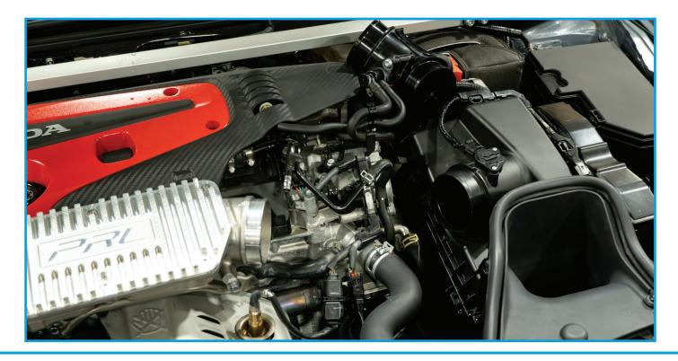
Remove the two 10mm bolts securing the upper turbocharger coolant feed line to the underside of the factory aluminum inlet pipe.
