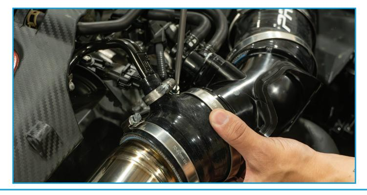
Securely tighten all the worm clamps. Once done, reinstall the two 10mm upper turbocharger coolant feed line bolts you removed in step #4.
