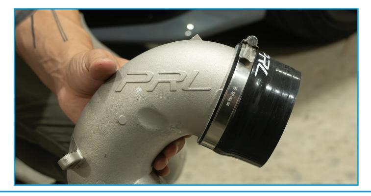
Make sure the surface of the Inlet Elbow that mounts to the turbo is clean and clear of any debris. Install the factory gasket onto this surface with the tabs wrapping around the flange as shows below.
