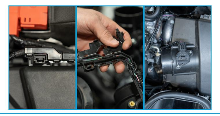
Remove the air box bolts holding the air box in the engine bay. There is one on the back side, one on the right side and two in front on the air box scoop. Pull the air box from the engine bay and set aside.
