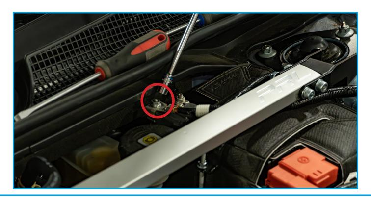
Loosen the 4 hose clamps on factory OE rubber connectors. Remove the valve cover vent hose from rubber boot connecting to OEM inlet pipe. Remove both the rubber connecting boots but leave plastic EVAP Purge Jet housing in the car.
