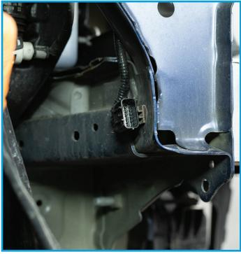
Remove the 6 plastic clips holding in the plastic splash tray underneath the factory intercooler. Remove this tray and set it aside.
