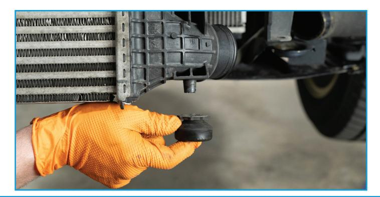
To make room for intalling the larger PRL Intercooler core, you will need to temporarily remove the fromt crash beam. You can do this by removing the 6 long 12mm bolts/nuts, 3 on each side of the beam. Set this all aside for now.
