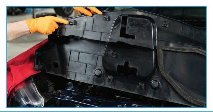
With the cover out of the way, you can now remove the 4 plastic clips holding in the top of the grill/bumper assembly. We recommend using a clip removal tool to prevent damage to any of these clips.
