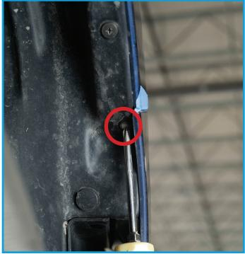
Underneath the car, you will need to remove all of the (6) plastic clips and (9) screws attaching the bumper to the underbody. Keep in mind that some of the screws are different (7x 10mm hex head, 2x phillips head)
