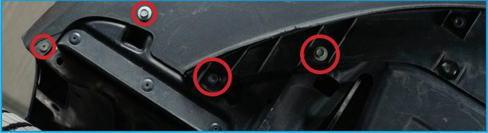
Finally, use a small flat head screw driver or plastic scraper to release the (6) tabs securing the bumper to the bottome of the headlight and fender. Repeat on both sides.
