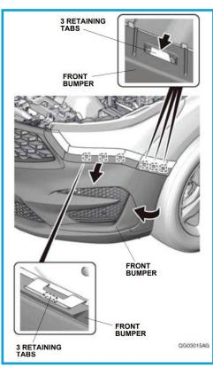
The bumper should nowbe free to pop off forwards. There is one electrical connector on the right side of the vehicle side that will still be holding the bumper to the chassis, so unplug this and carefully set the bumper to the side.
