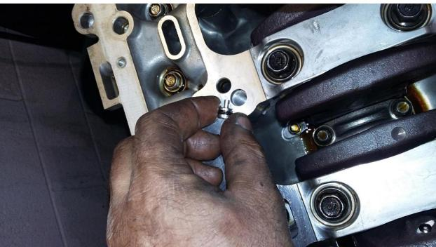
Using a 1/8" NPT tap, tap the main girdle and install the supplied 1/8" NPT plug into the oil jet port.
