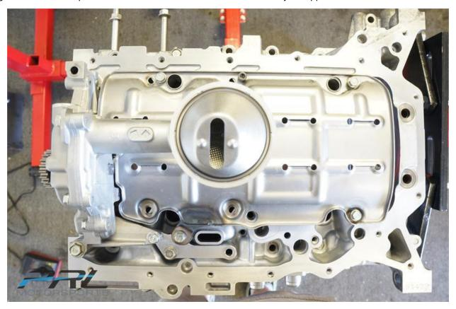
Assuming your engine is disassembled down to a bare block, we suggest starting with the initial modifications to the main girdle. Tap and block-off the small oil drain galley with the supplied 1/16" NPT plug.
