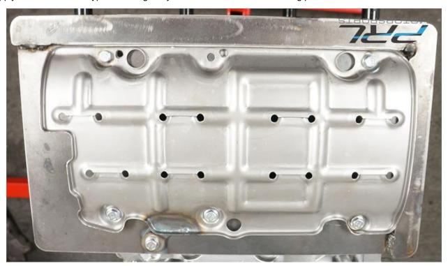
We suggest recessing two holes in the main girdle (opposite side to the oil jet) to utilize the two supplied 1/2" OD, 3/16" thick spacers to support, which attach the windage tray. Some customers and kits choose not to do this step, but we feel that not doing so allows for insufficient support and the possibility of rattling.
