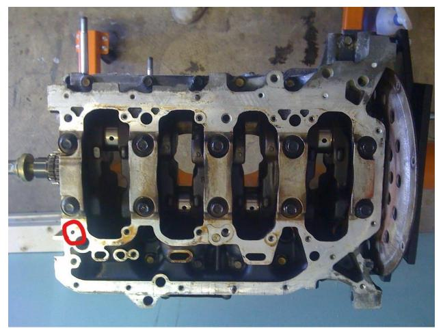
Located towards the center of the main girdle, remove the oil jet. This can be removed by threading in a self-tapping screw or using a pick to pry out. Be careful not to damage the girdle.
