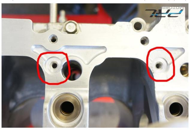
Install the oil pump mount using the correct length bolts.
