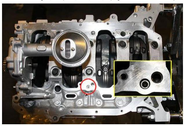
Below is how an unmodified PRB Type-S windage tray would fit to an unmodified K24Z girdle. Notice that only two bolts line up.
