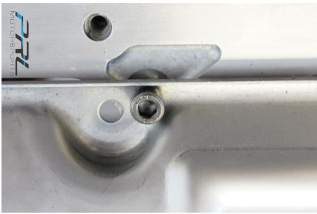
The factory K24Z oil filter housing can now be relocated (using the supplied oil filter relocation kit) to the top of the engine block where other K-Series utilize the oil filter housing.
