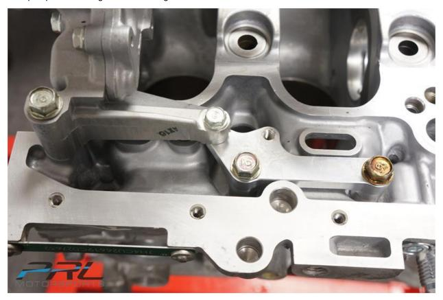
Making sure the main girdle is clean and free of all debris, the oil pump and windage tray can now be installed using a mixture of PRL and customer supplied hardware.
