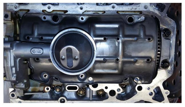
We supply a modified PRB Type-S windage tray to allow for additional mounting points.
