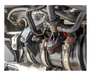
4. Release the intake duct from the shroud and the rubber connection between the intake duct and the airbox. This allows easier access to the airbox assembly.
