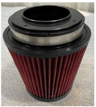
$12. \ Hold \ the filter \ and \ adapter \ assembly inside the airbox \ and \ align \ with the \ airbox \ inlet \ hole.$
