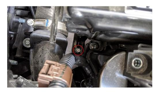
9. Pull the rubber grommet off of the standoff next to the fusebox, this requires quite a bit of force to remove, some leverage may need to be used with a pry tool. Insert this into the bottom of the PRL airbox.
