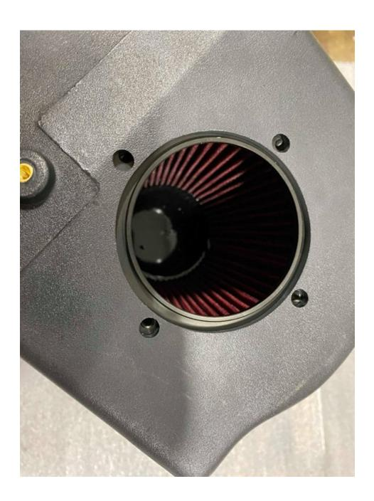
13. Place the MAF housing onto the adapter and secure using the 4 supplied M5x12mm bolts. Torque these bolts to 11.2 ft/lbs. This will "sandwich" the airbox in between both MAF components. With this connection the airbox acts as a crush washer seal.
