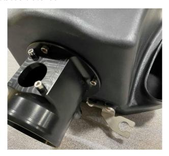
17. The bracket by the intake duct connection should be installed prior to placing the airbox in the vehicle as well.
