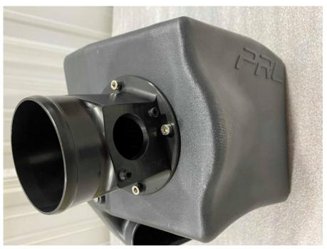
14. The filter should be secured to the adapter with gaps around each side of the filter for optimal performance. The filter should not be touching the inside walls of the airbox.
