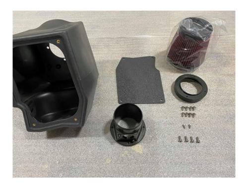
11. Remove bolts from airbox lid, remove lid. Pull out the packing material and remove filter from plastic packaging. Insert the machined MAF to filter adapter into the filter and tighten the hose clamp.
