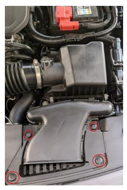
3. On the stock intake tube, loosen the clamps on each end, one connected to the airbox and the other connecting to the plastic inlet pipe. Remove the small hose clamp from the evap system, and the two bolts on the adapter section, one is behind the hose shown in the picture. Below shows an example of what the connection looks like.
