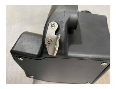
18. Both of the brackets utilize the factory rubber dampeners. Place them inside the bracket eyelet that houses them.
