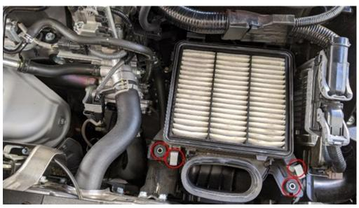
8. One final bolt remains on the side of the airbox, it is recommended to remove the ECU to provide better access. Or use a swivel head. If removing the ECU and reinstalling be sure to take extreme caution not to damage any pins, these are sensitive and important for the full operation of your vehicle. ECU's are expensive to replace!
