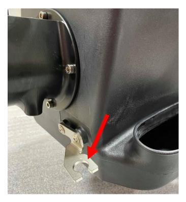
19. Place the MAF sensor in the PRL MAF Housing, connect the MAF sensor plug and secure using the PRL SUPPLIED BOLTS. **NOTE: The factory bolts will not work properly, they are a different length.** Keep your factory bolts in a safe place if reverting back to stock in the future
