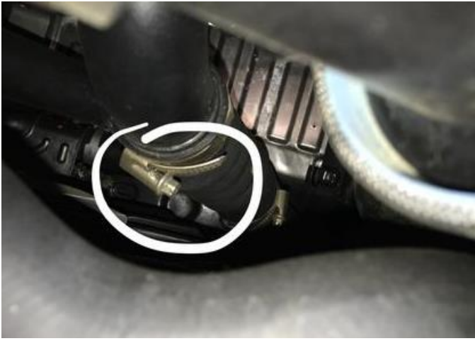
11. Disconnect the charge pipe on the driver side (from the top of the engine bay).
