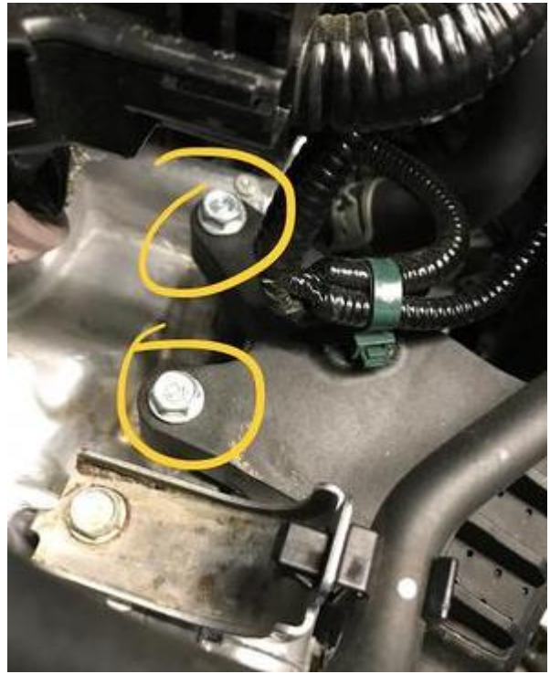
13. There are two bolts on the cold side charge pipe that secure the charge pipe to the engine, remove them
