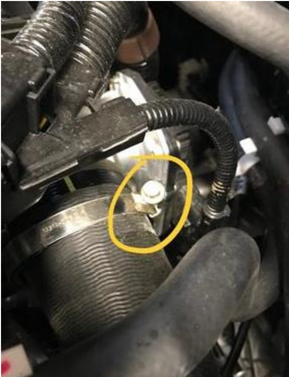
12. Disconnect the coupler at the throttle body between the firewall and the valve cover:
