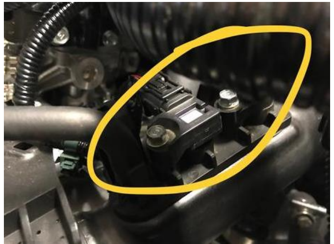
14. Carefully unplug the two sensors on the cold side charge pipe and remove the entire charge pipe.
