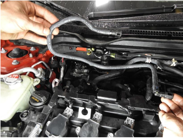
6. The completely removed fuel line:
