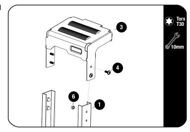
Loosely assemble the Ladder Rung
