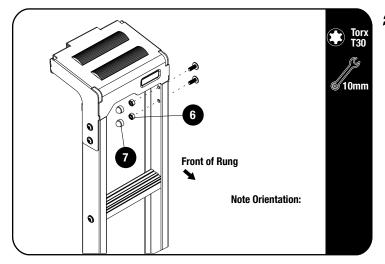
Fully tighten all Fasteners.
