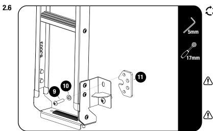
Secure the Ladder Hinge Mount Bracket to the hinge using M8 x 35 Button Head Bolts, M8 x 16 x 1.6 Flat Washers and the Hinge Spacer (Items 9, 10 & 11)
