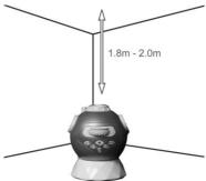
2. Place the unit over the stand (15) on a flat and stable platform (e.g. a table), the optimum project distance is about 1.8m to 2m.
