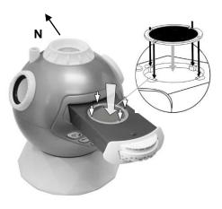
**3.** Press the Slide Tray Eject Button (7) to open the tray and install the star disc (16). Note the keys on the disc have to match the ridges on the tray.
