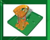
8. Attach the head bottom (7) to the front pole of the bottom
