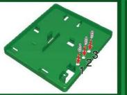
Connect the wires by bending the spring over to create a gap into which the metal wire is inserted: Slide switch red wires - 12 Battery holder red wire - 2 Battery holder black wire - 3
