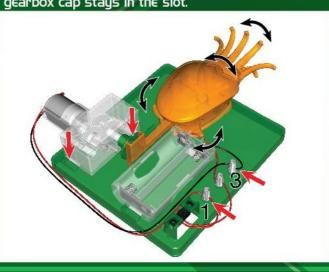
20. You're done! Insert the batteries (see "Battery Installation" section below) and push the slide switch to the right to see the robotic cuttlefish moves as indicated by the black arrows!
