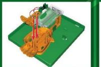
Install the arm plate (9) on the arms. The flat side should be faced inwards.
