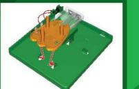
5. Install the fins (4) on rear pins of the base plate.
