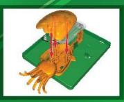
17. Insert the motor (15) into the gearbox (I3) until it is locked in position.
