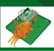
IO. Install three arms (5) by aligning its pins to the corresponding holes on the T-plate and the slots of the
