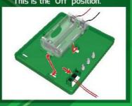
Install the support plate (2) on the base plate (II). Lock it into position by the hooks on the base plate.
