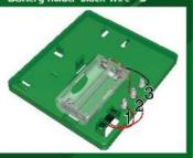
Install and lock the battery holder (I2) and slide switch (I6) in place as shown. Note the pin without wire is on the left.
