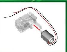
10. Cover the shaft of the gearbox (9) with the gearbox cap (II).
