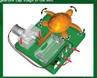
12. You're done! Insert the batteries (see "Battery Installation" section below) and push the slide switch to the "ON" position to see the robotic turtle swims as indicated by the black arrows!
