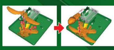
7. Fix the right angle arm (7) on the base plate (IS) with its pin inserted into the hole of the right hind flipper.
