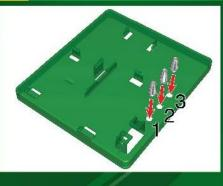
2. Install and lock the battery holder (8) and slide switch (12) in place as shown. Note the pin without wire is on the left. Slide the switch to the left. This is the "Off" position.
