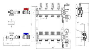
The balancing of the heang system is in compliance with BS EN1264-4. All flow meters can be connuously adjusted by simply rotang the glass tubes located at the top of the manifold.
