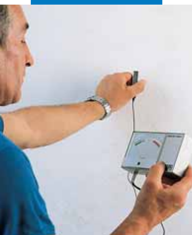
Checking plaster humidity
