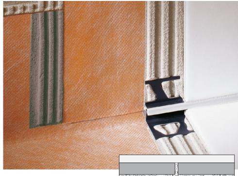
Schlüter®-KERDI-DS is a special polyethylene membrane for bonded waterproofing assemblies and serves as a vapour barrier with an s<sub>d</sub> value of more than 100 m, which is considered a vapour barrier in physical construction terms. The waterproofing membrane is 0.5 mm thick and equipped with water vapour blocking additives.
